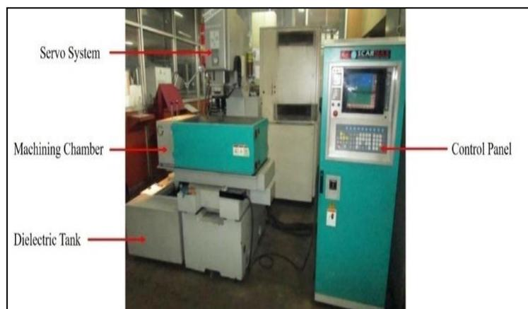
**Figure 1.** Electric Discharge Machining Setup
