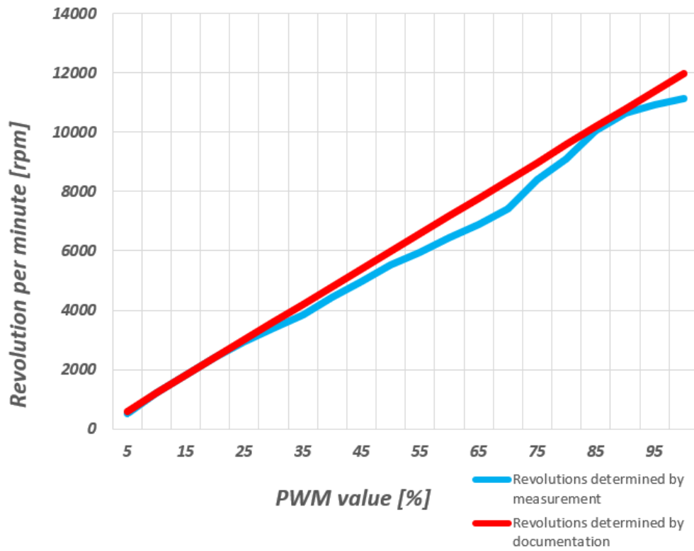
Figure 4. Ideal and calculated motor speed characteristics for PWM values, measurements carried out at 12.60V
