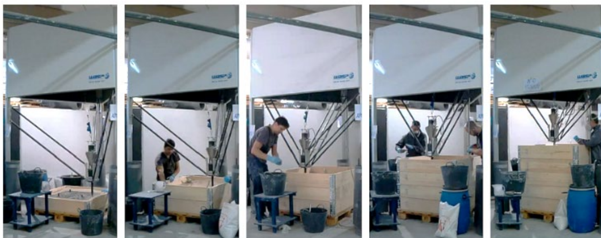
Figure 5. Sequence of manufacturing process using 3D printer [26]
