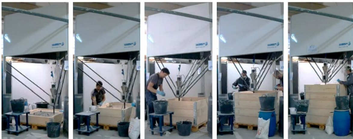
Figure 5. Sequence of manufacturing process using 3D printer [26]
