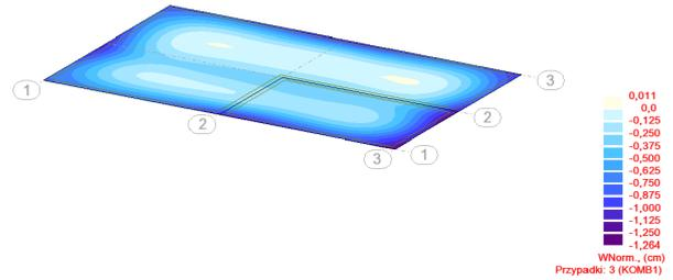
1. Figure 11. Map of the deflection of the foundation slab in the Z direction - variant II [13]
