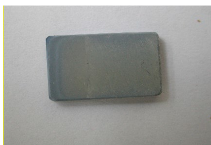
Figure 6. Surface of the sample before oxidation
