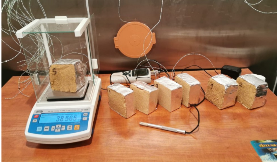
Figure 1. Measurement set inside the climate chamber
